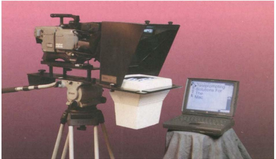
The prompting configuration used by Vidox Image and Data combines QuickPrompt software, a nine-inch VGA monitor, and a Vinten Vision 20 tripod.
