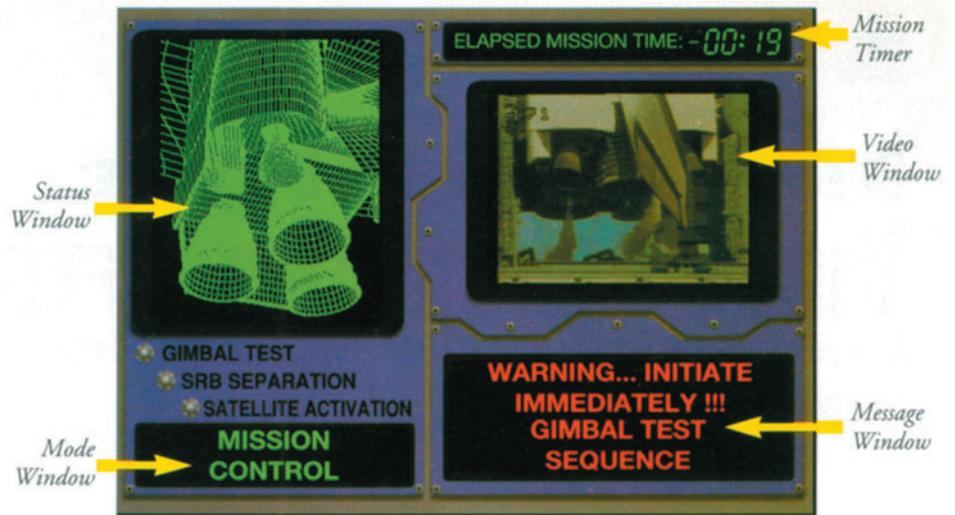
A typical Simulator screen, with all the elements of the interface marked.
