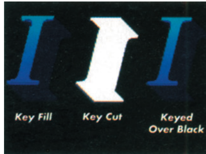
Key fill and key cut signals for the letter I, with and extruded drop-shadow. The edges of the key fill signal are jaggy, and the edges of the key cut signal are antialiased. Note that software antialiasing occurs within the key fill (where the edge of the letter meets its drop-shadow). Using the antialiased key cut signal, a linear keyer will blend the edges of the key fill with background video (enlarged 10 times normal size).
