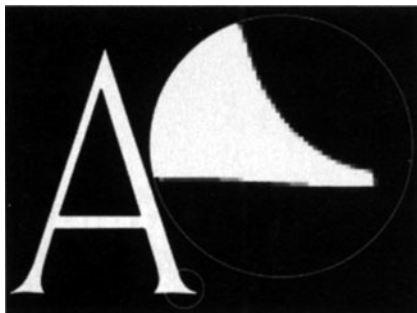
Antialiased character with close-up of serif. Note that the edges of the character blend from white to black.
